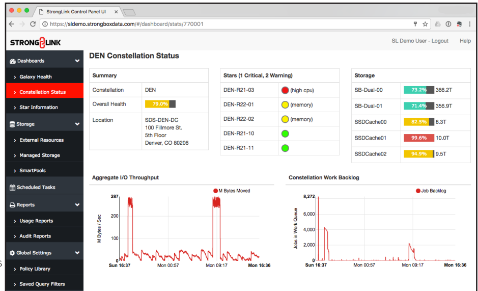
Fig. 4 - The StrongLINK control panel enables global management of storage and data policies. A rich reporting engine can automate utilization and audit reports across all storage types, to provide the intelligence needed to enable pro-active planning.
